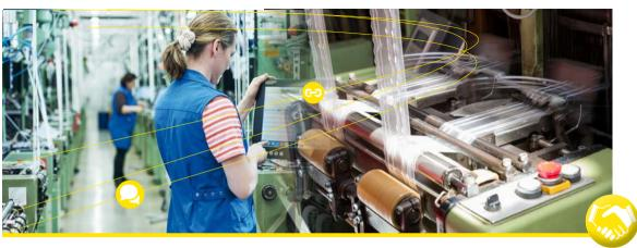
The machines were equipped with 10" touch displays, the usability of which was implemented in close coordination with the specifications already captured during the inventory process and the specific requirements of the machine operator. As we know from our experience in other projects, this personalization and individualization increases acceptance of the new and initially unfamiliar solution.
